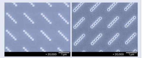
make nanoscale pits on the photoresist film, but that only shallow nanopatterns could be produced on the resist film because the nanopatterning depth is strongly dependent on the localized profile of the near-field light. He also emphasized that the patterns did not always directly reflect the photomask.
