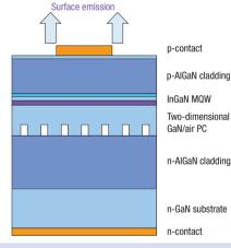
The laser consists of a layer of InGaN multiple quantum wells (MQW), which are grown over the top of a GaN/air two-dimensional photonic-crystal structure and surrounded by cladding layers and electrodes.
