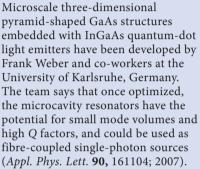
The resonators rely on internal reflection of light from the tilted pyramid facets to achieve strong confinement of light in all three spatial dimensions with low loss. The researchers fabricated the structures using a combination of molecular-beam epitaxy, electron-beam lithography and wet chemical etching. They report that the techniques allow versatile control of cavity shape, size and facet angle, as well as fabrication of more complex structures.
