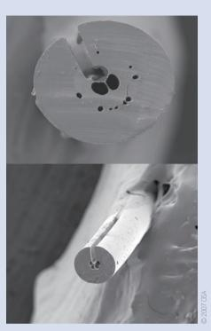
an analyte instant access to the core at any point along the fibre's length; signal light can be injected through a spliced conventional fibre.
