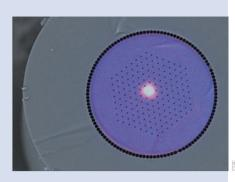
by using a double-clad photonic-crystal fibre with a large core and high numerical aperture to enhance nonlinear optical effects and signal collection. Although not yet observed, the team says that the approach is potentially promising for *in vivo* three-dimensional imaging of deep tissue, allowing tissue analysis without the need for extracting samples.
