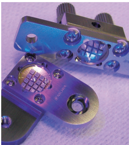
Nichia's 5 W 365 nm LED array module, which is now under development for applications such as inkjet printing and photolithography.
