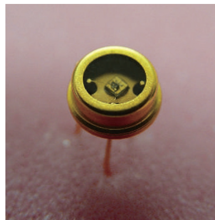
The UVTOP LEDs are allegedly the first AlGaN devices to offer wavelengths of 250 nm to 340 nm.
