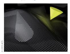
Scanning probe microscopes, such as the scanning tunnelling microscope (STM), are often used to reveal the morphology of a sample. With graphene, however, the sample will follow the tip rather than the other way round and images of graphene's surprisingly undulating landscape are dominated by tip-induced deformations. Jannik Meyer and colleagues at the University of Vienna have now been able to measure these deformations by using an STM set-up with two tips.
