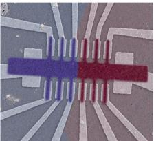
Chemical vapour deposition can be used to grow graphene films on the metre scale. These films are, however, polycrystalline and have numerous grain boundaries, which can scatter charge carries and adversely affect the electronic properties of the films. Jiwoong Park and colleagues at Cornell University and Columbia University have now shown that overlap between crystallites in such polycrystalline graphene can be used to improve the conductivity of the films.
