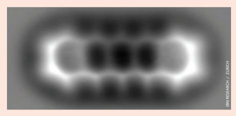
an AFM, and by probing the short-range chemical forces, Gross and colleagues were able to resolve the atomic positions and bonds inside the pentacene molecules.
