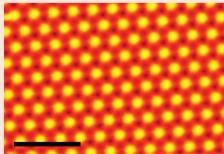
bar is 10 nm), whereas type-II films have a  $\sqrt{3} \times \sqrt{3}$  structure and a similar lattice constant to the silicon substrate (right). The films also have different transition temperatures — 4.9 K for type-I and 3.65 K for type-II — which the Texas team attribute to the type-II film experiencing tensile strain
