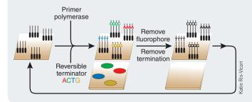
Sequencing with reversible terminators. Synthesis reagents, added to the flow cell, consist of primers, DNA polymerase and four differently labeled, reversible terminator nucleotides. After incorporation of a nucleotide, which is identified by its color, the 3' terminator on the base and the fluorophore are removed, and the cycle is repeated for a read length of 30-35 nucleotides.
