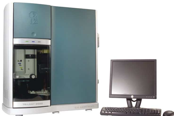
The Trilogy 2020 instrument from U.S. Genomics uses fluorescence correlation spectroscopy for the sensitive quantification of microRNA targets. (Courtesy of U.S. Genomics.)
