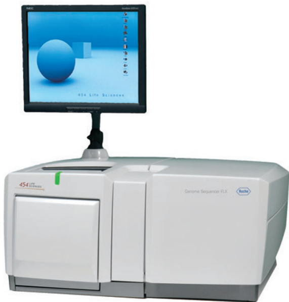
Figure 1 | The Genome Sequencer FLX instrument. The Genome Sequencer FLX supports a number of formats, allowing users to customize the number of samples per instrument run and the number of reads per sample. A single run can be physically divided into 2, 4 or 16 samples with 210,000 reads per sample, 70,000 reads per sample and 12,000 reads per sample.
