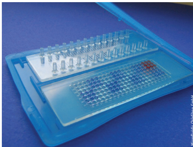
An example of the small scale of microfluidics as a microscopy slide often serves as the standard footprint for many microfluidic devices.
