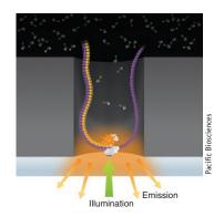
Individual polymerase molecules immobilized within ZMWs in an aluminum substrate generate detectable pulses as fluorescently labeled bases associate with the enzyme before their addition to the nascent DNA chain.
