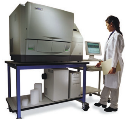
The Megabace 4500 system can generate 2.8 million bases in a 24-hour period. (Courtesy of GE Healthcare.)
