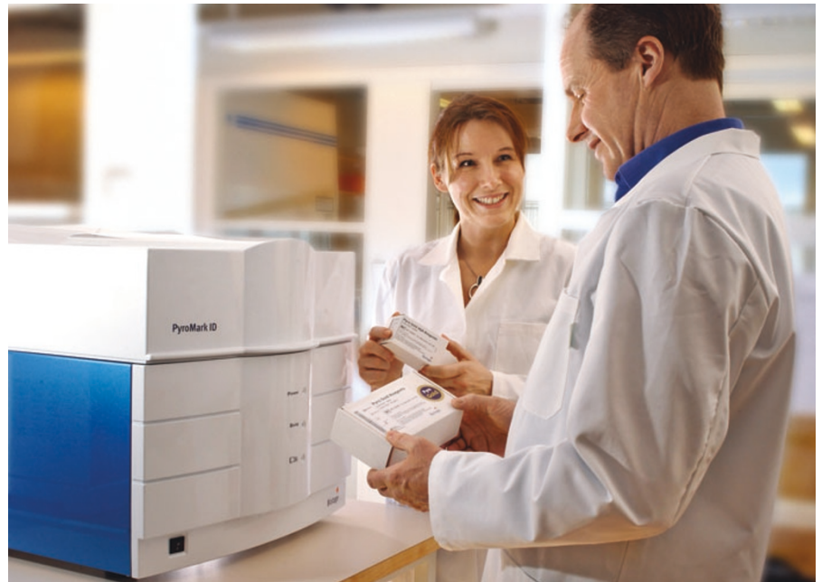
The PyroMark ID uses Pyrosequencing to read a DNA sequence. (Courtesy of Biotage.)
