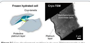
Figure 2 | A key development enabling *in situ* cryo-TEM tomography is the specialized FIB milling procedure enabled by the Scios DualBeam that removes sample material above and below the desired thin lamella. Adapted with permission from ref. 1.
