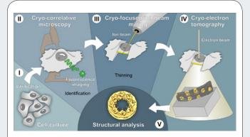
Figure 1 | The five essential steps of the cryo-TEM tomography workflow. Each step is supported by/within FEI's product portfolio/Workflow. Vitrobot (I), CorrSight (II), Scios (III), Titan Krios (IV), Amira (V).
