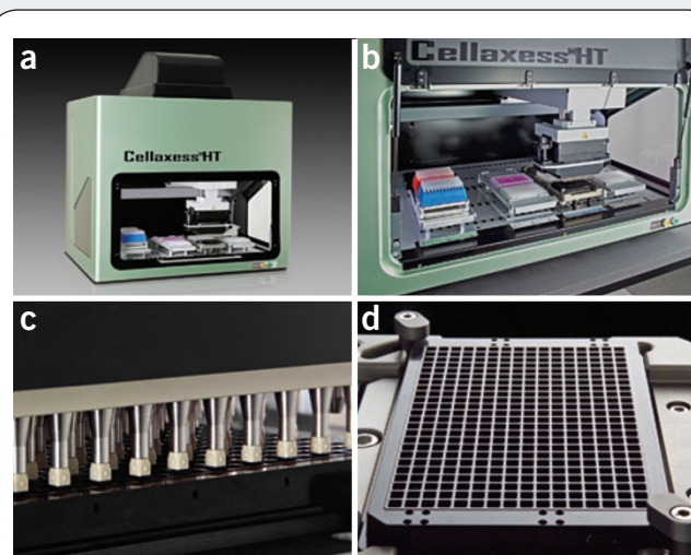
Figure 1 | Layout of the CellaxessHT system. (a) An overview of the system in stand-alone configuration. The HEPA filter unit can be seen on top of the system. (b) The deck layout during an experiment, the deck being loaded with the electroporation module, liquid handling tips, trays with electroporation buffer and culture medium, and cell source and control plates. (c) A close-up image of the capillary electrodes as they are approaching the CellaxessHT 384-well plate. (d) The plate.
