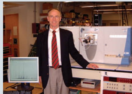
Don Hunt in front of the first mass spectrometer that performs electron-transfer dissociation, a technique for retaining post-translational modifications.
