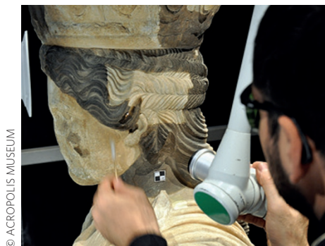
One of the Caryatids in the Acropolis museum, getting a facelift using a dual laser system developed for the project by the Acropolis Museum and the Institute of Electronic Structure and Laser at the Foundation for Research and Technology in Crete.
