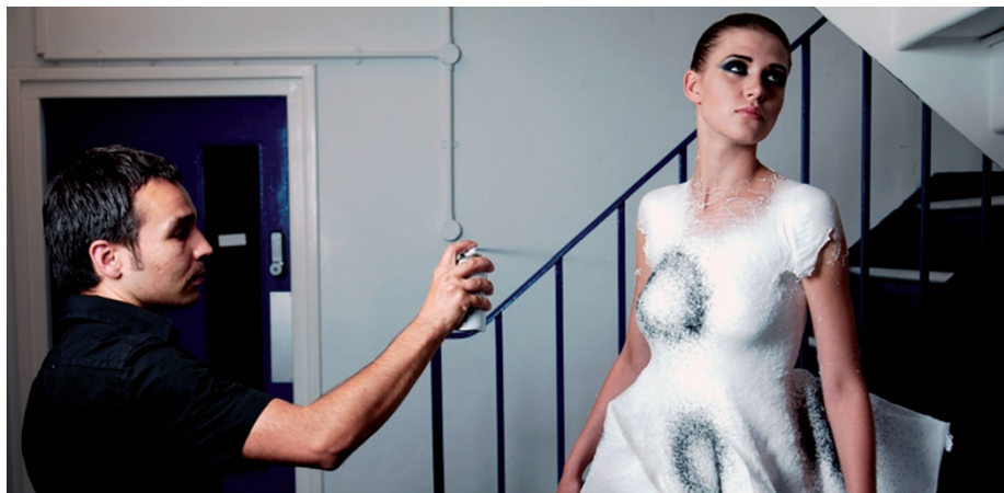
Figure 1 | Design and materials science meet. Dresses from aerosols by Fabrican ( www.fabricanltd.com ). Image by Gene Kiegel.
