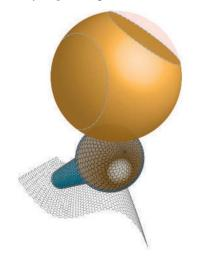
Dispensing zeptolitre droplets of gold–germanium alloy from a nanopipette allows crystallization in this size regime to be studied.
