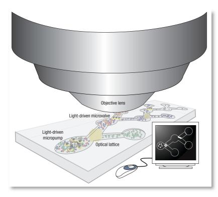
Figure 2 The 'lab-on-a-microscope' concept.
