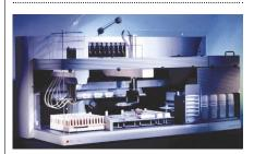
Tecan's workstation automates microplate-based assays.
