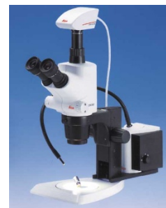
Stereomicroscope with 6.3:1 zoom capability.
