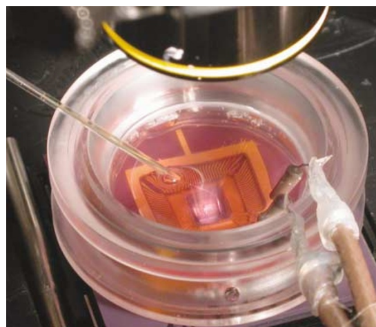
Bridging the gap: a neurochip, based on the work of Peter Fromherz, links biology and technology together.
