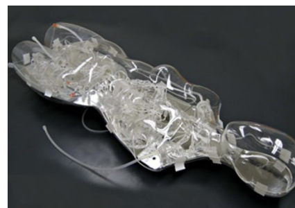
Eve, the endovascular evaluator. A mannequin for training, evaluation and simulation of endovascular surgery.
