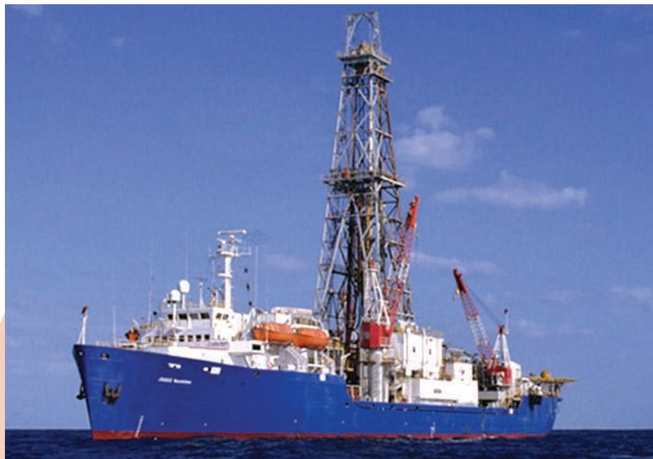
JOIDES Resolution : the drilling vessel used to obtain sediment cores from the sea floor in the northwest Pacific Ocean.
