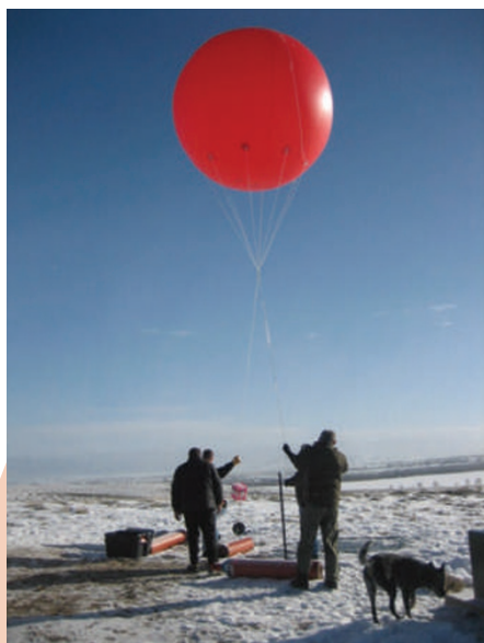
Balloon-borne ozonesonde used to measure vertical profiles of near-surface ozone during winter production events.
