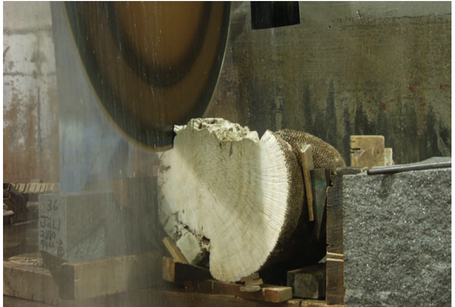
A coral around a metre across is sliced for sampling at a granite mine.
