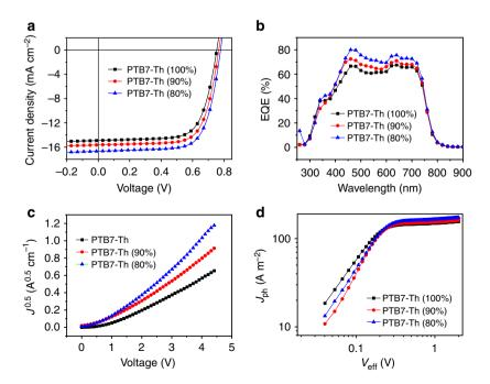
**Figure 2 | Photovoltaic performance of the ternary devices. (a)** Current density versus voltage characteristics of PTB7-Th:PID2:PC<sub>71</sub>BM with 0, 10 and 20% PID2 content. (b) EQE curves for the ternary devices. (c) Hole mobility for the ternary system. (d) Photocurrent density versus effective voltage curves.
