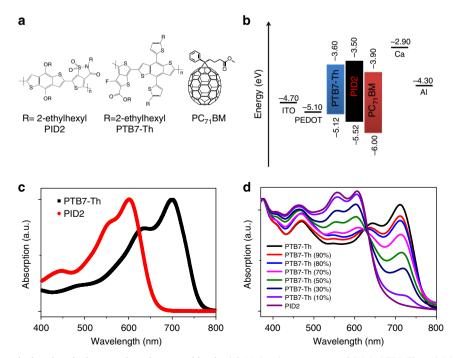
**Figure 1 | Structures, electrical and optical properties of ternary blends.** (a) Molecular structures of PID2, PTB7-Th and PC<sub>71</sub>BM. (b) Energy levels of materials used in the solar cell device. (c) UV-vis absorption spectra of PTB7-Th and PID2 in chloroform. (d) UV-vis absorption spectra of PTB7-Th:PID2:PC<sub>71</sub>BM films with different PTB7-Th:PID2 weight ratios.
