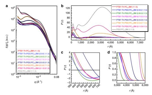
**Figure 4 | RSoXS characterization of the ternary films. (a)** RSoXS profiles (open symbols), calculated l(q) (solid lines), and (b) corresponding P(r) of PTB7-Th:PID2:PC<sub>71</sub>BM ternary systems. (c,d) The enlarged regimes of P(r) at the range of r = 350-700 Å and 3,000-6,000 Å, respectively.
