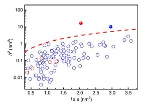
Figure 5 | Parameters of the graphene wrinkles studied in this work. The parameters, l and h, of both the graphene monolayer wrinkles (blue circles) and graphene bilayer wrinkles (red circles) studied in our experiment. The filled circle represents the wrinkles showing LLs and the open circles are denoted by the wrinkles that do not show any evidence of the LL. The red dashed curve is plotted according to  $h^2/la = 1$ .
