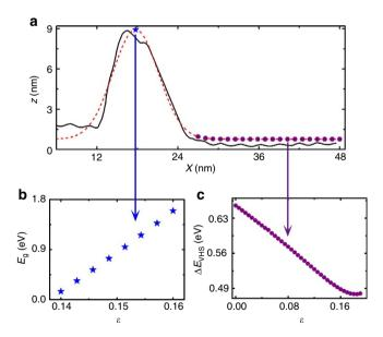
**Figure 4 | Energy gap and**  $\Delta E_{vhs}$  **as a function of strain.** In panel (a), the red dash line corresponds to a Gaussian fitting to the section line of the graphene wrinkle, as shown in Fig. 1c. Panel (b) shows that the energy gap increases as the strain increases for a fixed curvature radius of  $\sim$ 1.41 nm at the top of the wrinkle. Panel (c) shows the value of  $\Delta E_{vhs}$  as a function of the strain in flat twisted graphene bilayer.
