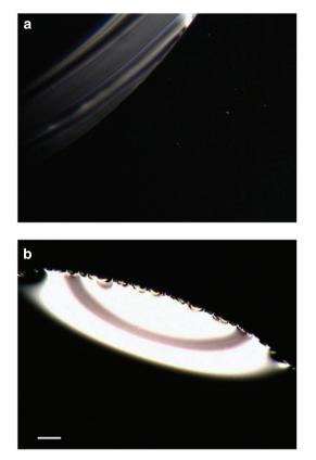
**Figure 4 | Images of water drops on silane-treated silicon and graphene.** Top view of a water drop on a (**a**) silane-treated silicon (**b**) graphene surface. The serrated three-phase line is evident on graphene, whereas on the non-graphene surface, the three-phase line appears smooth. The different light contrast corresponds to different light optimization for the different drop contact angles. Scale bar is 100 μm.
