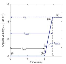
Figure 2 | Experimental procedure of a single-force datum measurement.
