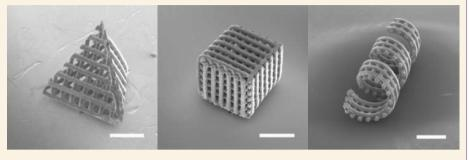
volatility. The printed, lattice-like sheets could be manipulated into complex 3D architectures that would otherwise not be possible to create through direct printing or lithography.
