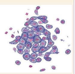
Subsequently, the team found that direct exposure to the electron beam disturbed the clusters, making imaging impossible, and so they turned to a technique commonly used for soft biological samples. This involved focusing the electron beam at an area adjacent to the cluster and imaging for a very short time in order to lower the dose of electrons. Images of nearly one thousand particles were taken and processed (three of the particle images are pictured, left) and
