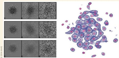
Subsequently, the team found that direct exposure to the electron beam disturbed the clusters, making imaging impossible, and so they turned to a technique commonly used for soft biological samples. This involved focusing the electron beam at an area adjacent to the cluster and imaging for a very short time in order to lower the dose of electrons. Images of nearly one thousand particles were taken and processed (three of the particle images are pictured, left) and
