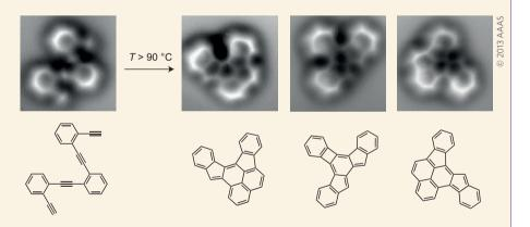
blob-like features present on the surface following the reaction suggested that a range of products are formed. Higherresolution images obtained using noncontact atomic force microscopy — in which the tip of the microscope is functionalized with a single CO molecule — revealed the different covalent-bond frameworks (pictured) of the molecules formed in a series of cyclization reactions.
