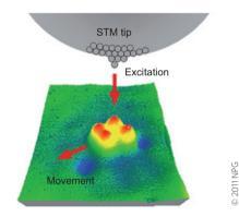
Single molecules can be pushed or pulled across a surface with the tip of a scanning tunnelling microscope (STM). Depending on their structure, some molecules will simply slide over a surface without changing their relative orientation, whereas others can be made to roll if the whole molecule, or parts of it, rotate with respect to the surface. In all of these examples, however, the molecule is a passive participant and goes along for the ride without being actively involved.
