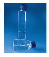
with angled neck allows easy access to the entire growth surface of the flasks with either a scraper or pipette. The flasks have either 25 or 75 cm<sup>2</sup> of growth area.
