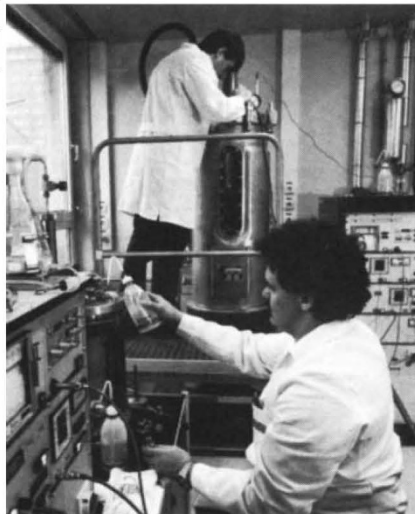
Chemie Linz moves into biotech: The 100-liter fermentor in the background is used to grow microorganisms for biological synthesis of organic materials.
