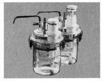
Agarpet $^{TM}$ , an adjustable dispenser, is an ideal tool for preparing agar plates easily and rapidly. It is autoclavable and designed to prevent contamination.
