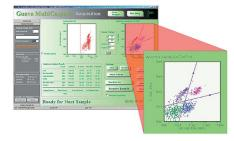
Guava Technologies' new assays allow users to easily gain a complete and highly quantitative profile of the stages of apoptosis. Designed to run on Guava's patented Guava PCA and PCA-96 cell analysis systems, they include assays for membrane changes (annexin V), activation of caspase enzymes and DNA fragmentation (TUNEL). The assays require only minimal numbers of cells, and include optimized reagent kits and easy-to-use software, in addition to the instrument used to analyze the cell samples.
