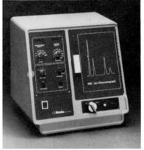
Brinkmann Instruments' (Westbury, NY) new Metrohm 690 ion chromatograph includes a high-pressure, low-pulsation pump, valve loop injector, column, and high-sensitivity (0.1 µS/cm) conductivity detector.
