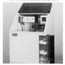
Designed to aid scale-up of protein or peptide separations, Septech's (Wakefield, RI) ST/800C preparative HPLC biochromatograph handles milligram to multi-gram sample loads. The system permits use of small (10 micron) packings in 1–3 in. diameter columns and includes a variable UV detector.
