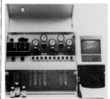
Porton Instruments' (Tarzana, CA) on-line HPLC interface connects the company's gas-phase protein sequencer with almost any HPLC system to divert part or all of an amino acid sample to the HPLC.
