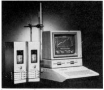
Isco's (Lincoln, NE) gradient controller for low pressure LC lets users automate binary gradient production and other functions of preparative and process-scale low pressure liquid chromatography for protein purification and other uses.
