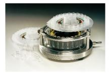
centrate target analytes and remove undesirable compounds, and this high-volume setup is five times faster than the manual syringe technique of preparing one sample at a time. The system comes with a manifold, sample carousel, and a specifically designed single-use filter plate containing 24 membrane filters.
