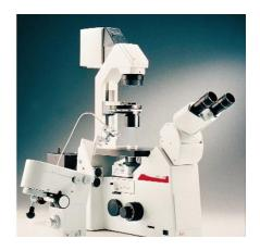
from Leica Microsystems (Deerfield, IL), is ideal for live cell research. Standard motorized fluorescence and a revolving filter turret for 0 pixel image shift make GFP time-lapse imaging and fluorescence colocalization studies easy to perform, and available options include a motorized objective nosepiece and focus, for accurate focusing of objectives down to 0.05 µm step sizes.
