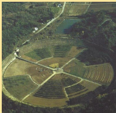
Part of the Atomic-GM facility at Institute of Radiation Breeding (Ibaraki, Japan). The gamma field has a radius of 100m and a 88.8TBq Cobalt-60 source at the center.
