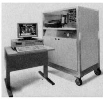
Process-Scale Chromatography The Kiloprep<sup>®</sup> 250 process-scale chromatography system from Biotage (Milford, MA) has a modular design and engineering features that allow a range of control, detection, flow-path, and column-technology options. Specifications include a flow rate of 0.1-1.1 L/min and an operating pressure of 2,000 psi.
