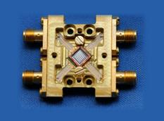
Superconducting detectors capture light at speeds not possible with conventional charge-coupled devices.
