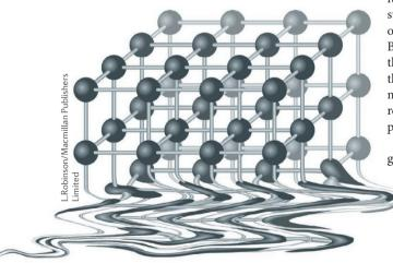
example of an intrinsically porous liquid — a 'MOF liquid'. When crystalline ZIF-4 is heated above its melting point (~865 K) and then cooled to room temperature, a melt-quenched glass is obtained. On heating to 856 K, the structural changes in this glass, as observed by X-ray diffraction, are consistent with the formation of a liquid.
