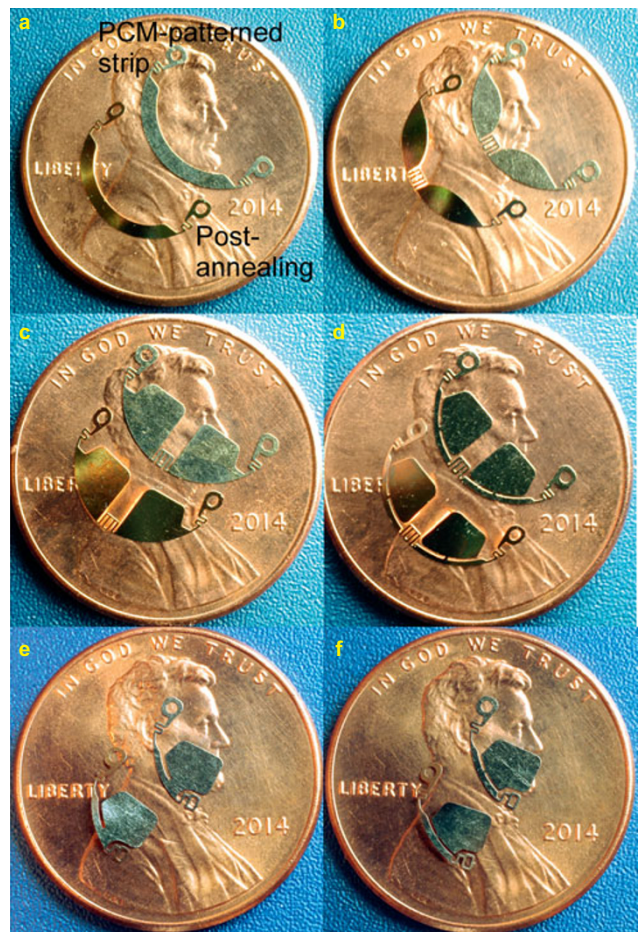
Figure 6 Fabricated actuators after photochemical machining and annealing: (a) Type A, (b) Type B 1 , (c) Type B 2 , (d) Type C, (e) Type D 1 , and (f) Type D 2 .
